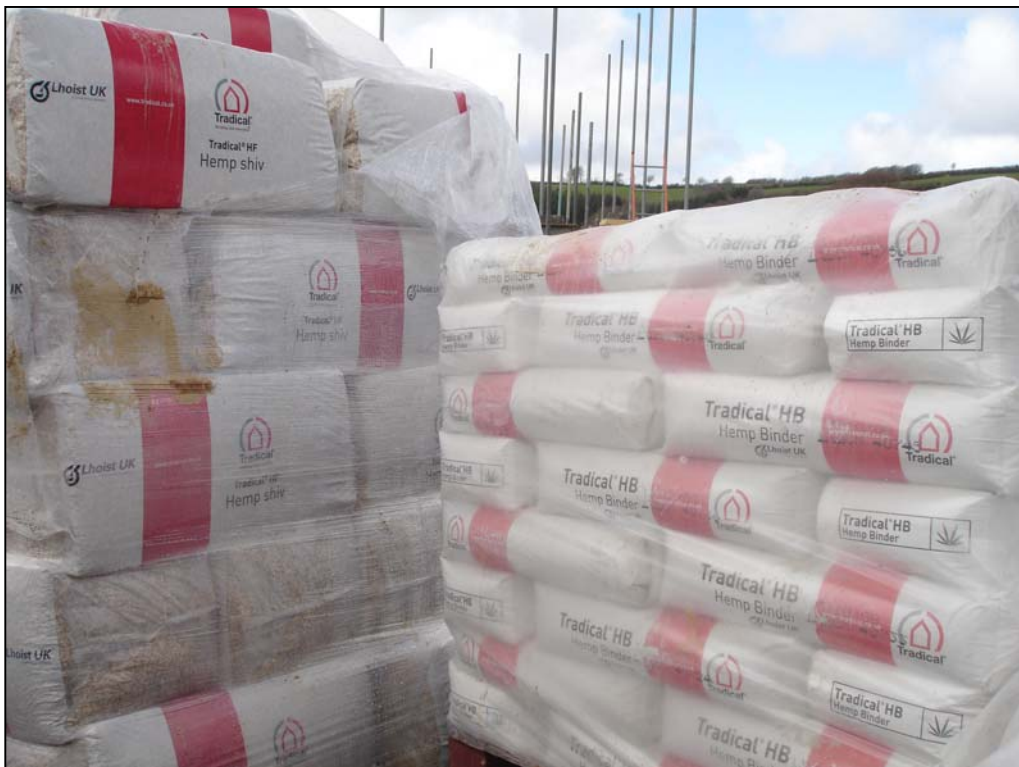
Figure 4. Hemp shiv and hemp binder for producing hemcrete.
