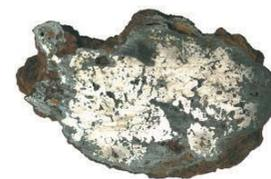
Cut and polished: a section through an iron bloom showing the solid metal and slag. Scale in mm
