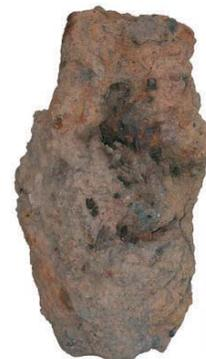
The curious case of the 'frozen' smelt: the contents of a failed furnace. Scale 20cm
