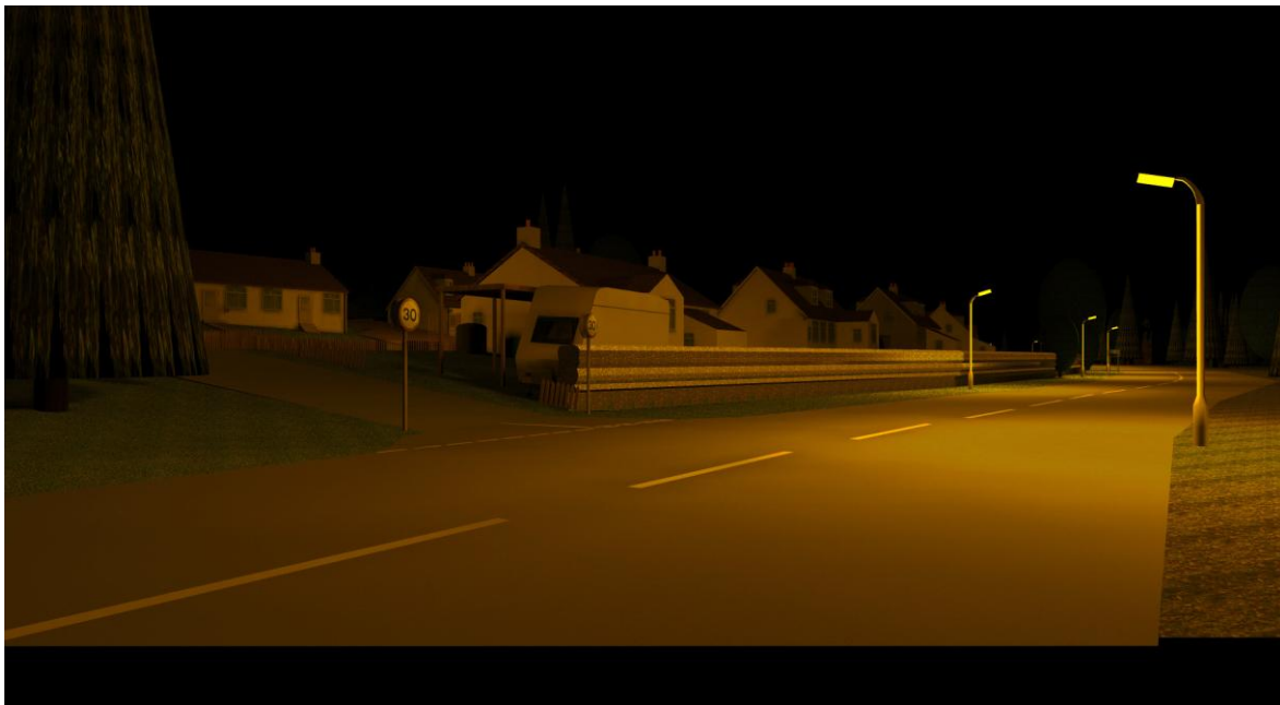
Figure 2.5 Traditional Low Pressure Sodium distribution - shows house details up to chimney pots
