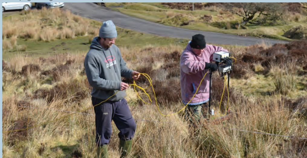
Different equipment is required to carry out resistivity survey
