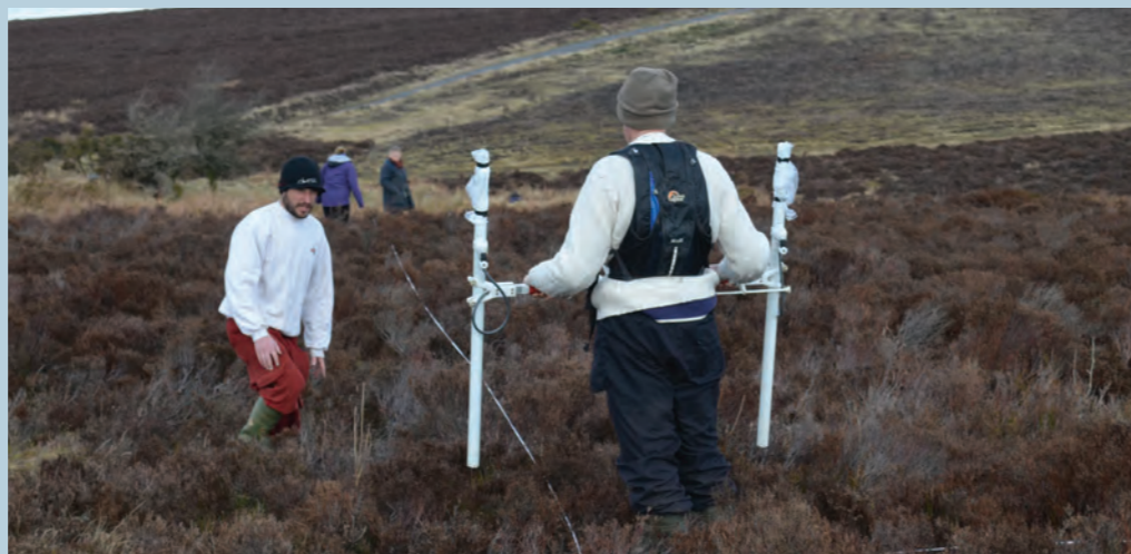
Carrying out a gradiometer survey at Hawkcombe Head
