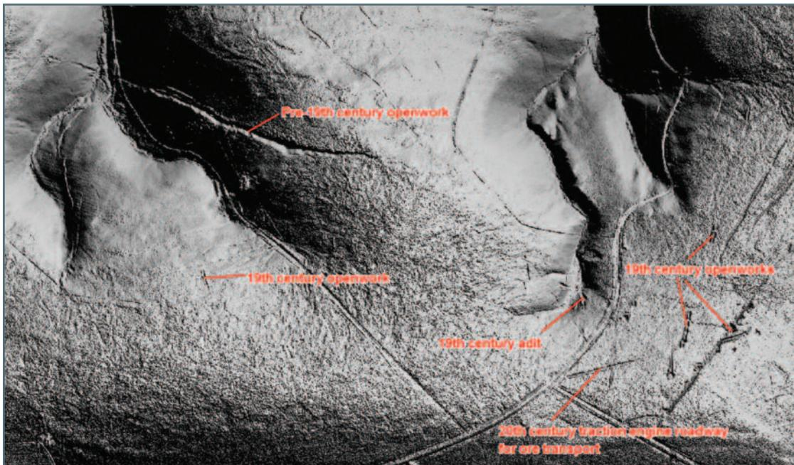
Figure 4: LiDAR digital terrain model showing the mining landscape on Burcombe and Deer Park.
