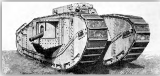
Mark VIII tank in World War I. It was 10m long, weighed 37 tonnes and travelled at 11 km/h
